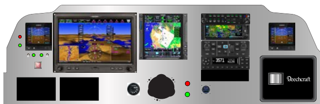
Figure 5: Panel Rev 3 – remove the 7" G3X display, move the GTN and second IFR GPS
