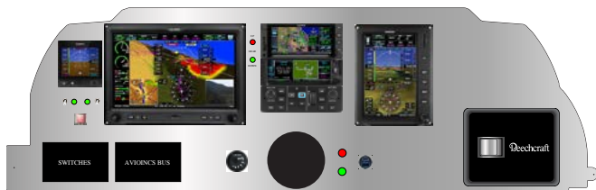
Figure 6: Panel Rev 4 – creative compromises, more capability in less space
