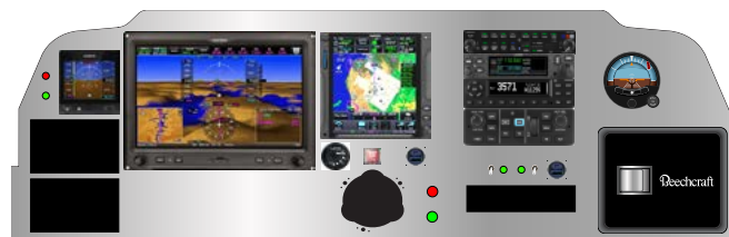
Figure 7: Panel Rev 5 – back to the GTN 750, keeping the legacy electric AI
