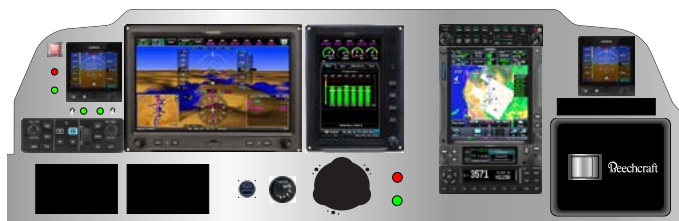
Figure 4: Panel Rev 2 – ergonomic improvements, GSB-15, and cubby added
