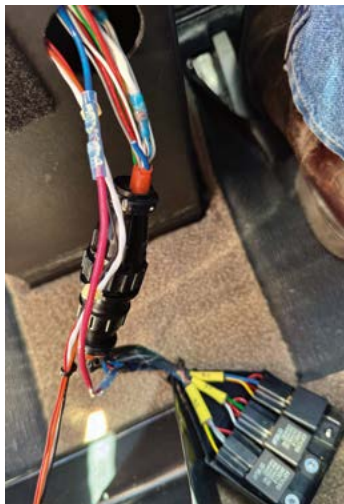
Photo 4: The splice on the FTA harness, bypassing pin 15
