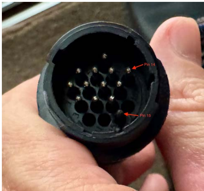
Photo 1: The relay module connector with the damaged pin 15 and the populated pin 14
